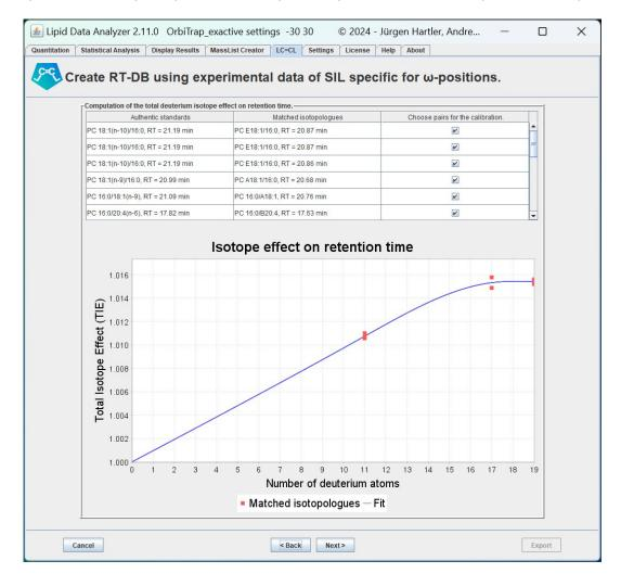
The tool fits a curve to enable interpolation for potential missing data points, i.e. SIL for which a suitable unlabeled authentic standard is unavailable.
