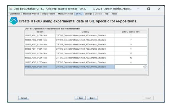
Upon loading and processing the data, you will see the panel displayed below. Each authentic standard is matched its labeled isotopologue. This step is crucial for the quality of the resulting RT-DB, as it determines the accuracy of the correction for the isotope effect on chromatographic retention. In this panel, you can manually verify the consistency of data points and correct for potential false positives.
