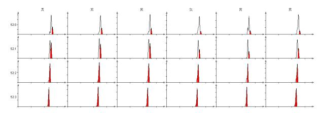
This picture shows a chroms export of TG52 of the LDA. It can be easily seen that analytes with more double bonds elute slightly earlier. This is a reliable quality criterion that the algorithm selected the correct hit.
