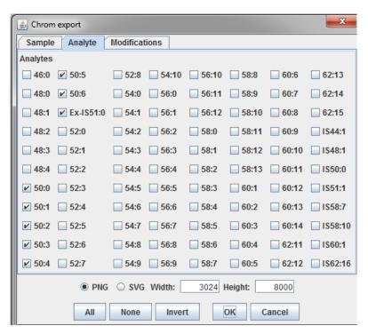
It is recommended to export just one or two lipid series at once. The chroms export can take some time, depending on the data and the amount of selected hits. The progress of the export is presented in a progress bar underneath the heat map.
