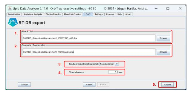
Panel (3.) allows for the optional adjustment of the isotope effect on chromatographic retention for the gradient. This is typically not required. Example files for this step can be found in the installation directory in the folder "gradients".
