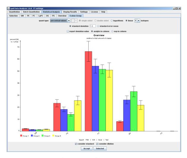
This overview has the option to "consider standard" (the current standard settings are taken) and to "consider dilution". If the "consider standard" is selected, an overview is displayed containing the standards used. If for one lipid subclass no standard is available, the subclass is neglected (like here LyPC). Without the "consider standard", these subclasses would have been displayed. Attention: without the "consider standard" it is assumed that all subclasses ionize equally!
