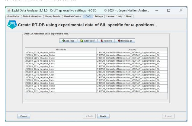
First, the RT-DB generator asks to enter LDA result files of SIL experiments as shown in the screenshot above. After loading and processing the data (with "Next >"), a panel to manually define which  $\omega$ -positions the individual stable isotope labels (denoted with different prefixes in the LDA result files) correspond to. In the current example (shown in the screenshot below), the "Label ID"/prefixes are defined as follows:
