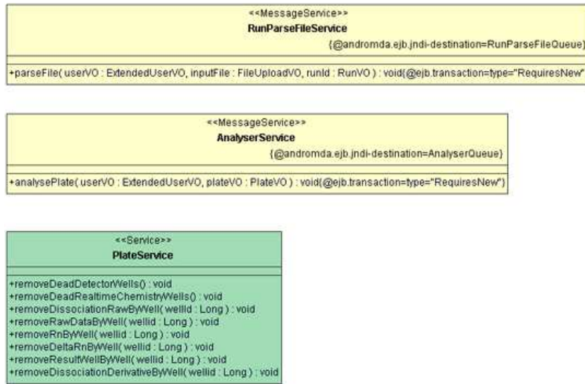
Figure 5.6: Shown are the three major services used in the developed application.
