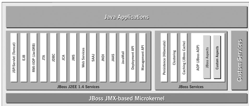
Figure 3.3: The JBoss Architecture [51]: The services JBoss provides, like the web server, security, persistence, etc. are registered with the microkernel and can be used by the web applications deployed in JBoss.
