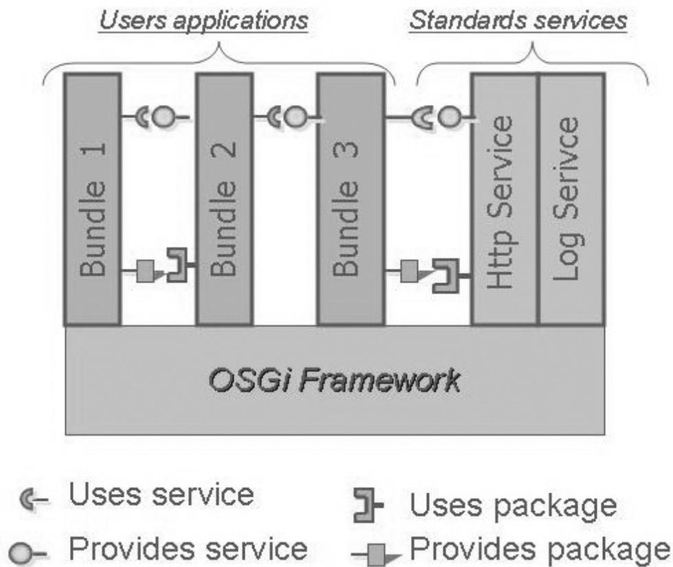
*Figure 2.1: The OSGi Architecture [36]: An OSGi application consists of bundles which can export and import packages and services.*
