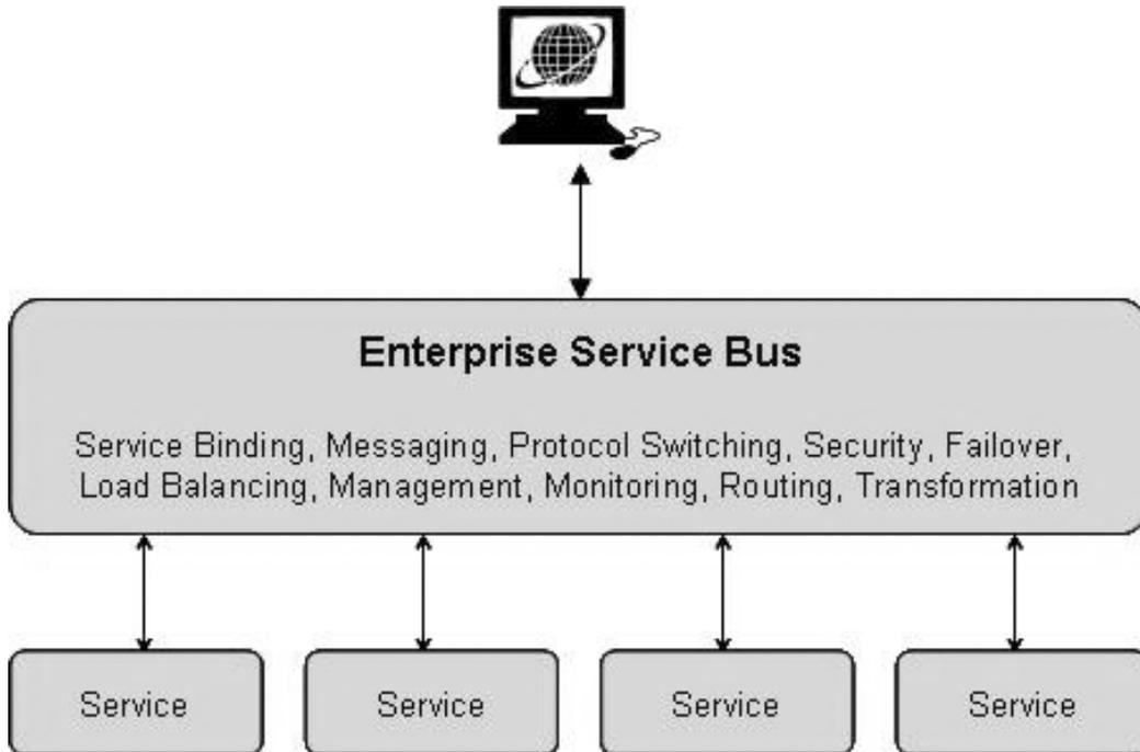
*Figure 2.2: The ESB Architecture [38]: Applications are connected to a common pipe through which the data is sent and which takes care of routing, transformation etc.*
