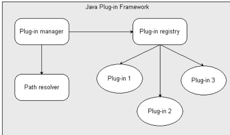
Figure 3.1: Java Plug-in Framework [44]: All the plugins are registered in the plugin registry. The plugin manager locates the code of the plugins with the help of the path resolver and then loads the code when the client requests it.
