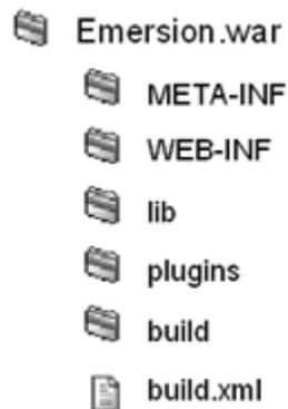
*Figure 4.2: Structure of Emersion.war: The `WEB-INF` folder contains the listener and the `web.xml` file. Various libraries are contained in the `lib` folder. The `plugins` folder contains the plugins and the `build` folder contains the compiled plugins. The `build.xml` file is used to compile the plugins and to copy the plugins from the `plugins` folder to the `build` folder.*
